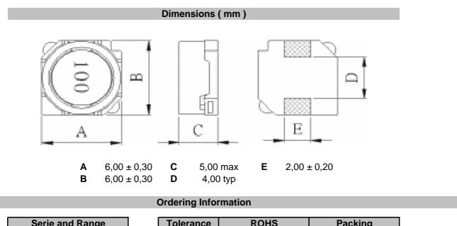
Serie and RangeToleranceROHSPackingS49004-151MRTRK = 10%R = ROHSBU = Bulk WareM = 20%N = non ROHSTR = Tape Reel
