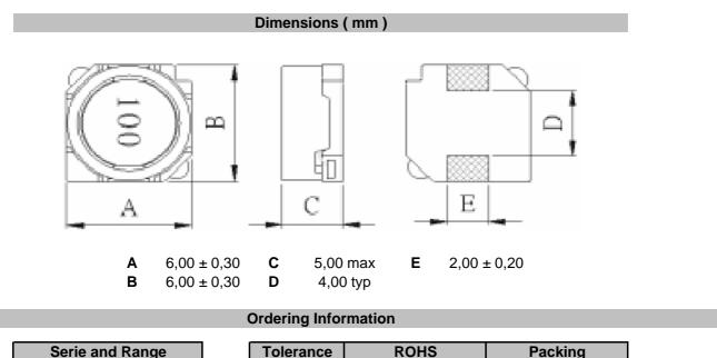
Serie and RangeToleranceROHSPackingS49004-150MRTRK = 10%R = ROHSBU = Bulk WareM = 20%N = non ROHSTR = Tape Reel
