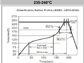
**Soldering Profile for Lead Free Soldering**
