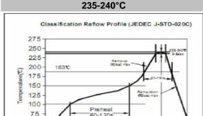
**Soldering Profile for Lead Free Soldering**
