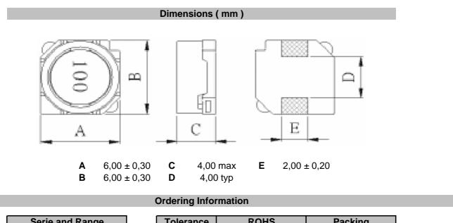
Serie and RangeToleranceROHSPackingS49003-121MRTRK = 10%R = ROHSBU = Bulk WareM = 20%N = non ROHSTR = Tape Reel
