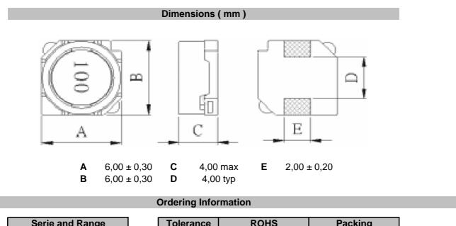
Serie and Range ROHS Packing Tolerance S49003-120 Μ R TR **K** = 10% R = ROHS BU = Bulk Ware **M** = 20% N = non ROHS TR = Tape Reel
