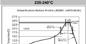
**Soldering Profile for Lead Free Soldering**
