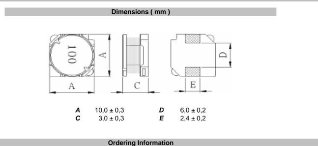
Serie and Range ROHS Packing Tolerance S46006-6R8 TR Μ R **K** = 10% R = ROHS BU = Bulk Ware TR = Tape Reel **M** = 20% N = non ROHS
