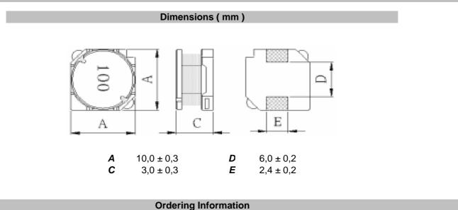
Serie and Range ROHS Packing Tolerance S46006-561 TR Μ R **K** = 10% R = ROHS BU = Bulk Ware **M** = 20% N = non ROHS TR = Tape Reel
