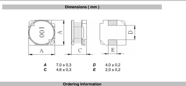
Serie and Range ROHS Packing Tolerance S46005-561 TR Μ R **K** = 10% R = ROHS BU = Bulk Ware TR = Tape Reel **M** = 20% N = non ROHS
