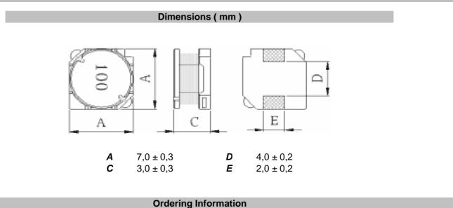
Serie and Range ROHS Packing Tolerance S46004-560 TR Μ R **K** = 10% R = ROHS BU = Bulk Ware **M** = 20% N = non ROHS TR = Tape Reel
