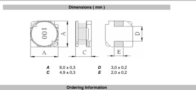
Serie and Range ROHS Packing Tolerance S46003-6R8 TR Μ R **K** = 10% R = ROHS BU = Bulk Ware **M** = 20% N = non ROHS TR = Tape Reel
