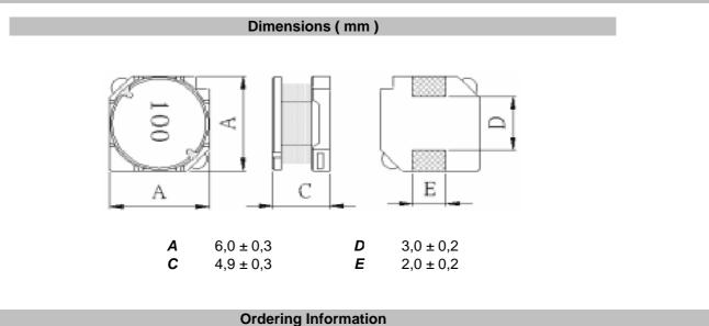
Serie and Range ROHS Packing Tolerance S46003-330 TR Μ R **K** = 10% R = ROHS BU = Bulk Ware TR = Tape Reel **M** = 20% N = non ROHS
