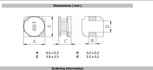
Serie and RangeToleranceROHSPackingS46002-681MRTRK = 10%R = ROHSBU = Bulk WareM = 20%N = non ROHSTR = Tape Reel
