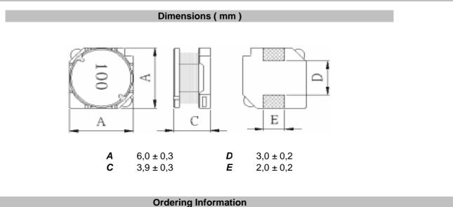
Serie and Range ROHS Packing Tolerance S46002-390 TR Μ R **K** = 10% R = ROHS BU = Bulk Ware **M** = 20% N = non ROHS TR = Tape Reel
