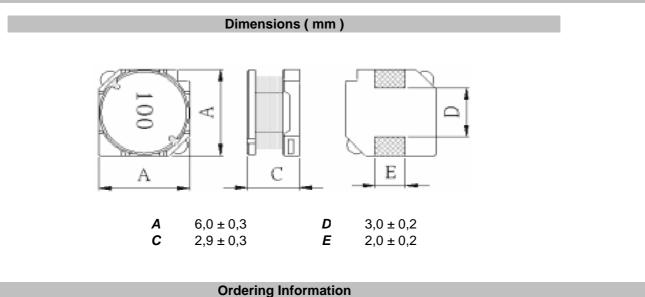
Serie and Range ROHS Packing Tolerance S46001-330 TR Μ R **K** = 10% R = ROHS BU = Bulk Ware **M** = 20% N = non ROHS TR = Tape Reel
