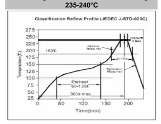
**Soldering Profile for Lead Free Soldering**
