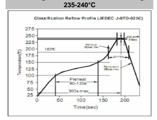
**Soldering Profile for Lead Free Soldering**
