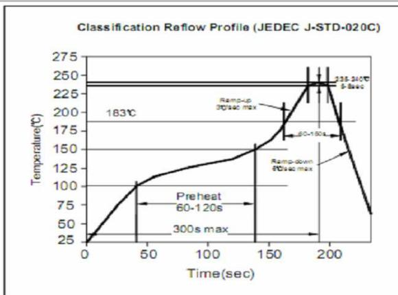
**Soldering Profile for Lead Free Soldering
